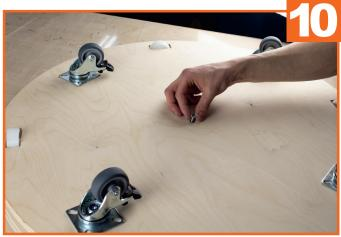
Screw F has to be mounted from the bottom of the Twister Plate into the thread.
